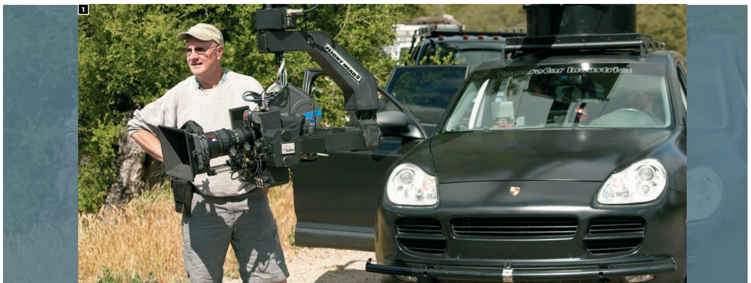
1 Bill Bennett, ASC with Camera Car Industries' Porsche Cayenne camera car rigged with a Filmotechnics Flight Head and Gemini Crane. (Photo Michael Helms)
